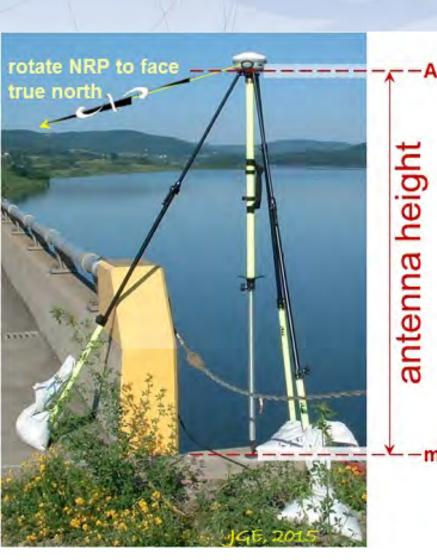
The height is measured vertically (NOT the slant height) from ARP the mark to the ARP of the antenna.
