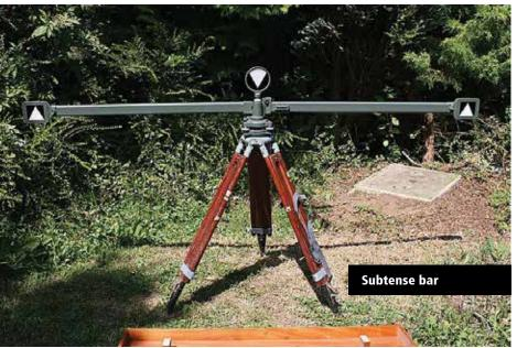
the tripod top until the sight tube was centered on the instrument operator. This would put the length of the subtense bar perpendicular to a line between the subtense bar and instrument.
