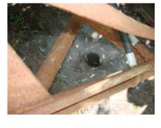
tripod on the loader frame to see if that would work. After some effort it was perched atop the arms and braces. The tribrach was leveled and focused and the iron rod came into view, just missing the east edge of the cross arm.
