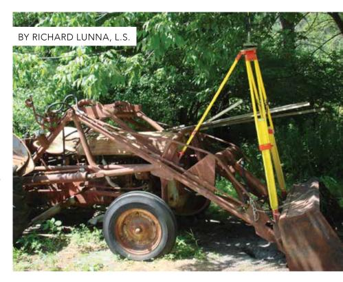
Unfortunately, the corner was located under the bucket loader cross arm so we couldn't use a prism pole to shoot it in. We tried again with the iron bar to move the tractor. No luck. We finally decided to set up a
